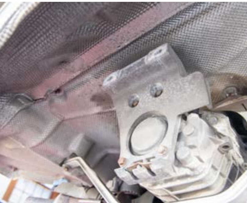
Muffler attachment bracket, see the holes all the way at the top!
