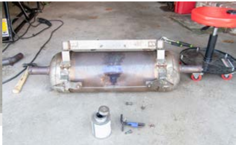
Bracket and repaired vibration dampers finally on!
