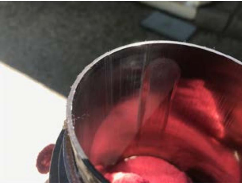
The groove let the pressure from the chamber above to escape and instead of providing power to move the car it pressurized the crankcase forcing oil vapor out the breather. The poor car looked like it was panting at idle. A new barrel and new clips solved the problem. That was a bigger job than most but still an easy fix.
